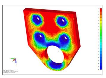
This detail shows the minimum principal strains for a metal bracket with bolt preload and contact surfaces.
